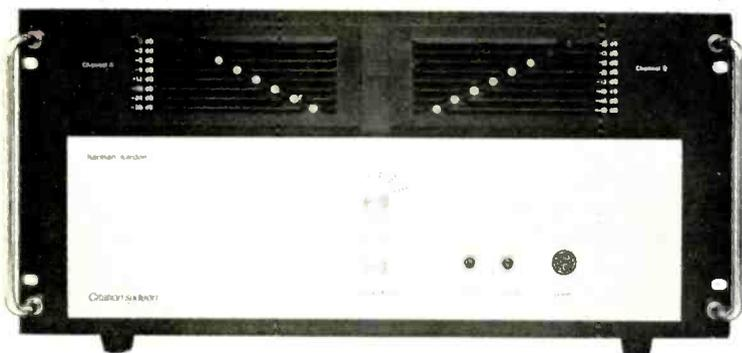
Output indicators for power amps are in, and Harman-Kardon uses an all-LED display for the purpose on Citation Sixteen.
