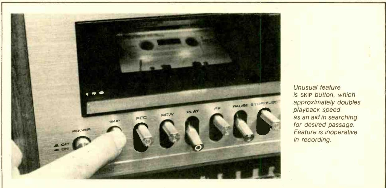
*Unusual feature is SKIP button, which approximately doubles playback speed as an aid in searching for desired passage. Feature is inoperative in recording.*
