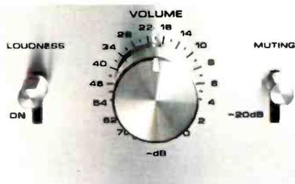
*Click-stop volume control calibrated in decibels, with left/right tracking within 0.5 dB.*
