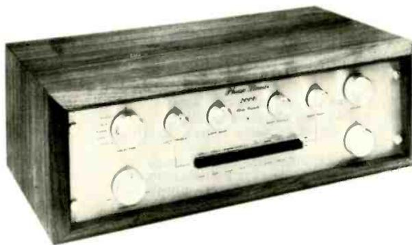
**The Equipment:** Phase Linear Model 2000, a stereo preamplifier/control center, in metal case with optional walnut case. Dimensions: 5½ by 19 inches (front panel), 6 inches deep, plus clearance for controls and connections. Price: \$299; walnut case, \$37. Warranty: three years parts and labor. Manufacturer: Phase Linear Corp., 20121 48th Ave., W. Lynnwood, Wash. 98036.
