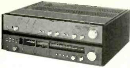
The unit is rated at 100 watts (20 dBW) per side, uses MOS FET output transistors, and has foil-type capacitors in place of electrolytic or ceramic devices. With an optional set of rosewood side panels, the amp can be paired with a Tandberg tuner to make a thoroughly deluxe "receiver." Shown here are the T1A-3012 amp (\$995) joined to the TPT-3001 tuner, for a total price (including side panels) of \$2,090.
