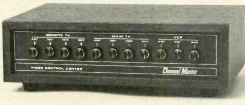
Channel Master's Video Control Center is a four-in/three-out RF switcher.
