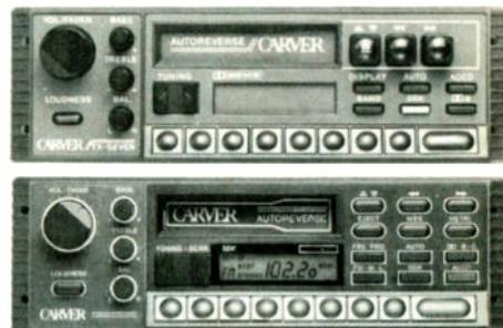
Naturally both decks are metal tape compatible with Dolby<sup>®</sup> noise reduction and have auto-reverse transports, separate bass, treble, balance and loudness and four-way fader controls. All tuning and transport functions are signalled with a gentle "beep" that keeps your eyes on the road, not on the compact, ergonomically-styled deck.
