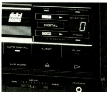
THE FRONT-PANEL DISPLAY OF THE CLD-909 SHOWS ONLY CHAPTER OR TRACK NUMBERS, RESPECTIVELY, FOR LASERDISCS OR CDs. A CONNECTED MONITOR SHOWS ADDITIONAL CUEING INFORMATION.
