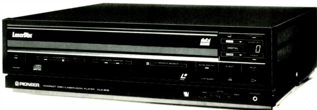
Laserdisc recess. You must slide it onto the tray, and there's not much room between the upper surface of the disc and the edge of the tray opening. Undoubtedly this inconvenience was necessary to reduce the height of the player.
