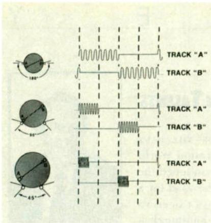
FIG. 3. THE USE OF DIFFERENT HEAD-DRUM DIAMETERS IN DAT PRODUCES THE VARIOUS HEAD-OUTPUT PATTERNS SEEN AT THE RIGHT (30 MILLIMETERS IS THE STANDARD ON THE FIRST GENERATION OF DAT DECKS). DIGITAL MEMORY CIRCUITS HELP TURN THE OBVIOUSLY DISCONTINUOUS NATURE OF DAT RECORDING AND PLAYBACK INTO CONTINUOUS AUDIO SIGNALS.
