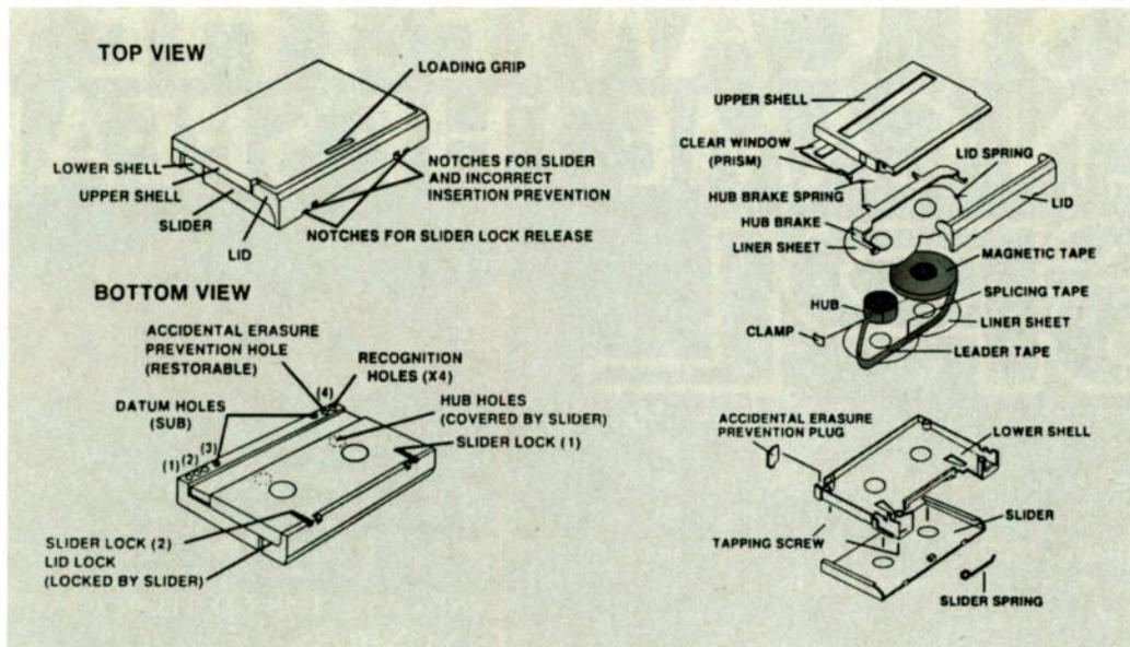
FIG. 1. THESE DIAGRAMS, COURTESY OF SONY, SHOW HOW FORM IS DETERMINED BY FUNCTION WITH A DAT CASSETTE. THE COMPLEXITY OF THE DESIGN ORIGINATES IN THE NEED TO KEEP THE TAPE DUST- AND FINGERPRINT-FREE.
