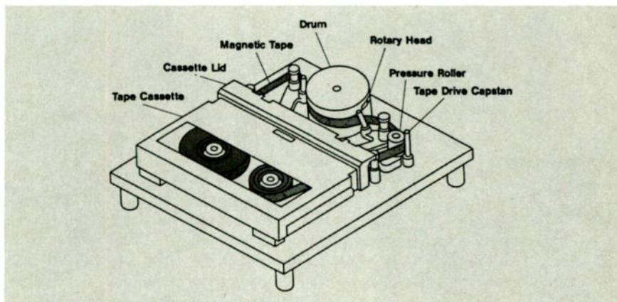
FIG. 2. THIS THUMBNAIL SKETCH OF A DAT LODGED IN A SIMPLIFIED HELICAL-SCAN MECHANISM SHOWS HOW THE TAPE IS DRAWN OUT OF THE CASSETTE AND WRAPPED AROUND THE SPINNING HEAD DRUM.
