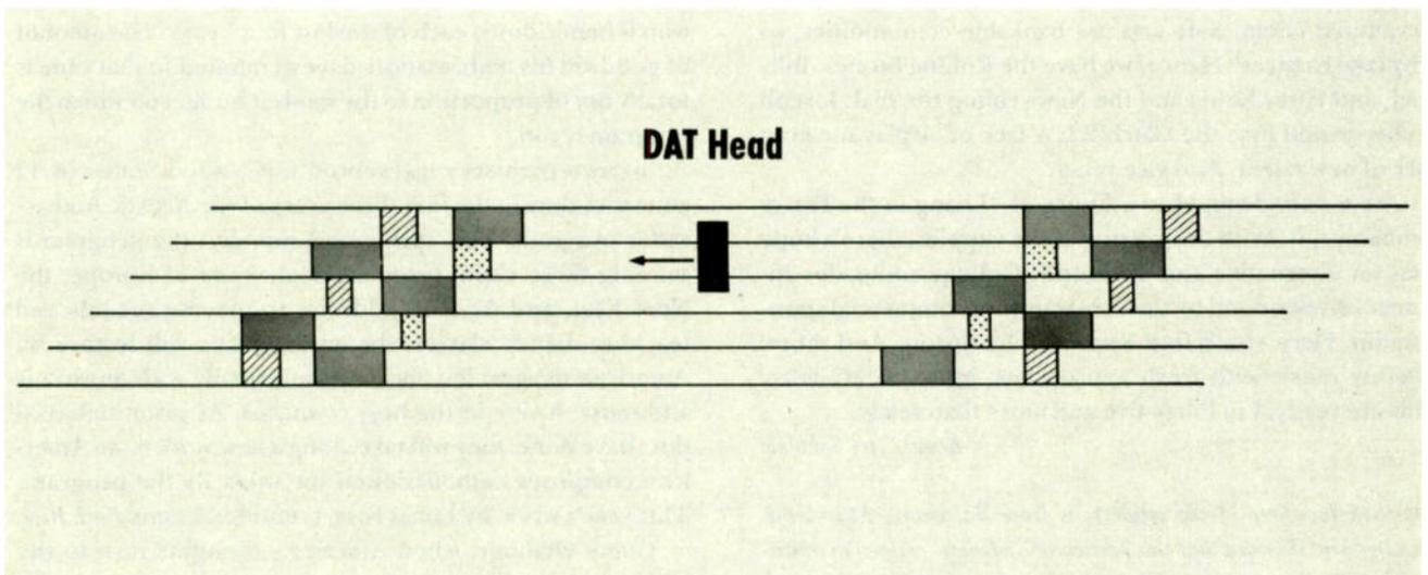
FIG. 4. EACH SUCCESSIVE TRACK CREATED BY A SPINNING DAT HEAD HAS A PATTERN OF PILOT AND SYNC FREQUENCIES DIFFERENT FROM ITS TWO NEIGHBORS. SINCE A DAT HEAD SPANS 1.5 TRACK-WIDTHS, IT PICKS UP PILOT AND SYNC SIGNALS FROM ADJACENT TRACKS, AND THESE IN TURN ARE USED TO CENTER THE HEAD OVER ITS INTENDED TRACK.
