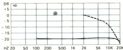
Relative output vs. frequency (at -20 dB)
