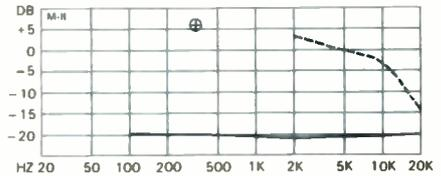
Relative output vs. frequency (at -20 dB)
