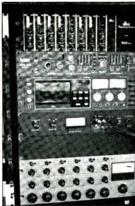
*Figure 6: The second equipment rack contains (top-to-bottom): 2 dbx Model 903 compressor/limiters (backing vocals and DI bass), and six Model 904 noise gates (floor tom, rack tom, guitar submaster bus, acoustic grand, and two spares); Lexicon Prime Time DDL (lead vocals); TEAC C-3 cassette machine; custom-built unit for monitoring AC line voltage, and console stereo left/right output selection; and an unused effects mixer.*
