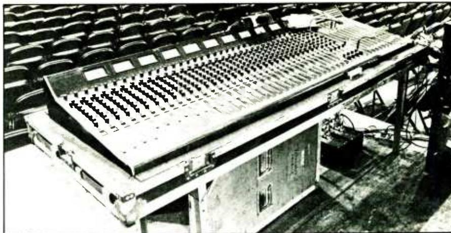
Figure 6: Midas 32-input PR Series stereo house console. Effects and outboard units also located at the house mixing position include a Roland SRE555 Chorus Echo, GML/Nova Research Model 8045 five-way stereo crossover, GML/Nova Series II Dynamic Gain Control compressor-limiters, Eventide H949 Harmonizer, Orban Model 622B parametric equalizer, Nakamichi 550 cassette and a ReVox B77 stereo reel-to-reel.
