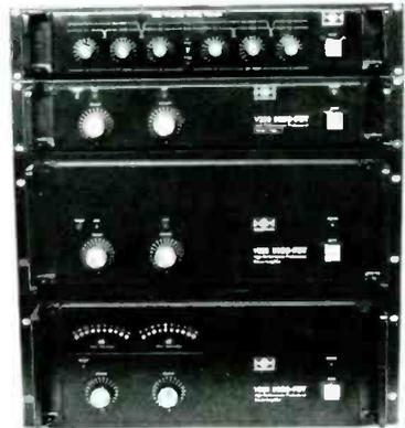
power amplifiers are short-circuit, open-circuit, and mismatch proof, and are unconditionally stable into highly reactive loads.
