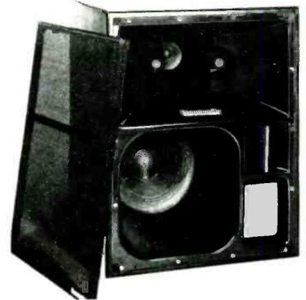
Frequency response is 45 Hz to 18 Hz,  $\pm 4$  dB; power handling 200-watts; sensitivity 101 dB 1 watt/1-metre full range, and 104 dB voice band.
