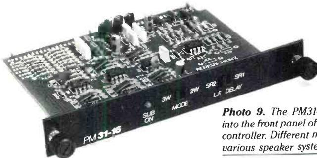
**Photo 9.** The PM31-15 circuit module plugs into the front panel of the Renkus-Heinz system controller. Different modules are available for various speaker systems.
