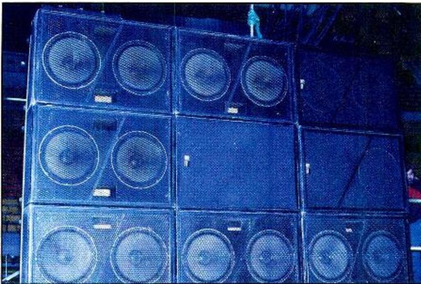
**Photo 13.** Large-scale concert use requires speaker system components that can fill huge performance spaces. Shown here, Meyer Sound Laboratories' 650-R2 subwoofers as fielded by Ultra-Sound at Meadowlands Arena in New Jersey.
