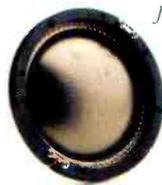
*JBL's 2450J Neodymium Compression Driver with Coherent Wave™ phasing plug provides in-phase combining of sound waves for extended high frequency performance. JBL's patented diamond surround titanium diaphragm with new embossed dome greatly reduces distortion and damage at high SPL.*
