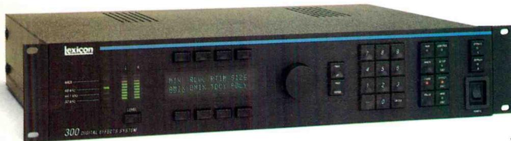
reverb and ambience. It automates sound changes with SMPTE/EBU time code. And it inputs and outputs analog, as well as consumer and professional digital formats — in any combination. All with magnificent Lexicon Sound.
