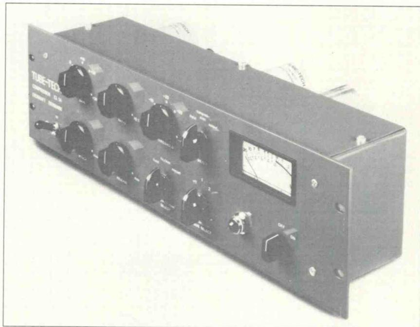
transformer and is controlled by side-chain amplifiers. Following the GRE is an all-tube push-pull amplifier with a wide gain range.
