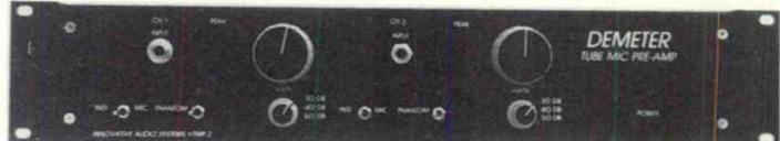
ALL TUBE DESIGN, TWO CHANNELS OF JENSEN 13K6C MIC TRANSFORMER INPUTS AND INSTRUMENT LEVEL INPUTS, PHANTOM POWER, VARIABLE GAIN, LOW THD (.06%), LOW NOISE (124 EIN), REASONABLY PRICED
