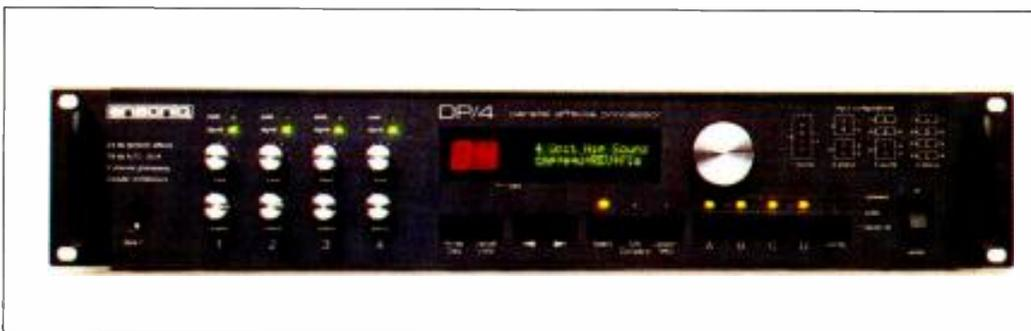
shift, with or without active panning, compression, EQ, DDL, reverb, rotating speaker (with inertia control!), tube guitar amplifier, tunable speaker, pitch shift, etc., etc., etc.
