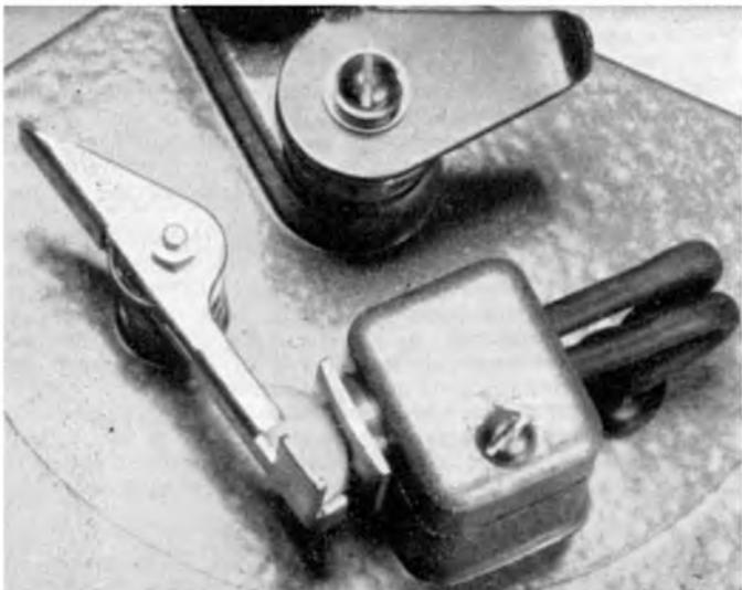
This close-up photo shows (top) the swing-back catch which permits the tape to be dropped into the channel for erase. The permanent magnet erase head is beneath the screw. (Bottom), the tape head, with the pressure pad which can be swung back by finger pressure on the arm.
