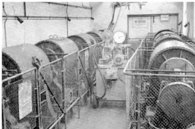
Fig. 2—Ball mills thoroughly separate the minute particles.
