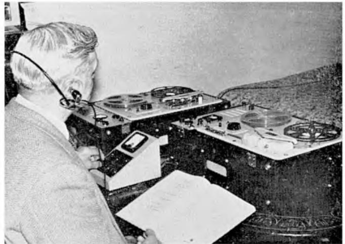
fessionally, because they could be erased. However, they are a boon to the amateur, and give a far superior reproduction to the optical track. It is now possible to have an optical sound track made from a magnetic sound track if a large number of prints are required. The only way to copy a magnetic sound track is to re-record from it.
