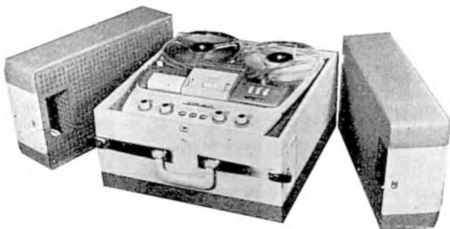
input source. Output connections are available for two stereophonic channels or monophonic signal and for Extension Loudspeakers. There are facilities for superimposition and a Temporary Stop Control is fitted. Control is by push-button. The TK.60 is remarkably compact, and is contained in the now well-known Grundig blue-grey case. The price is £134 8s.
