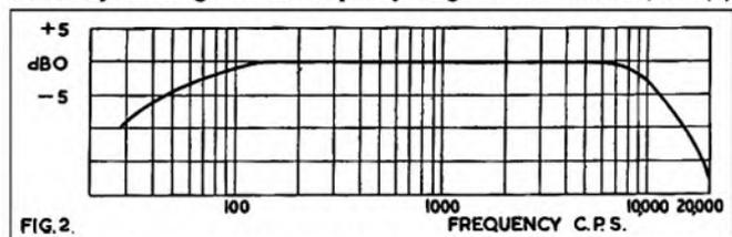
without indicating the loss at these frequencies, can be appreciated from fig. 2, which might be claimed as "3 dB down at 60 and 10,000 c/s," " $\pm 3$  dB between 40 and 12,000 c/s," or "response from 20 to 20,000 c/s."
