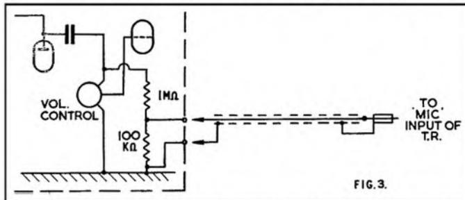
Fig. 3: The "diode" connection goes to the microphone socket.
