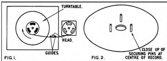
Fig. 1 (Left) Using the take up spool on a gramophone turntable to pull the tape past the head. Fig. 2 (Right) Securing pins may be fused or drilled into an old disc, to give firm drive of the spool.
