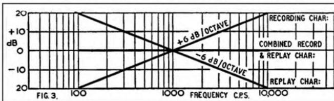
Fig. 3: Combination of rising and falling graphs to give flat response.
