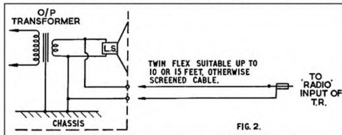
Fig. 2: The correct way to use Ext. L/S terminals.
