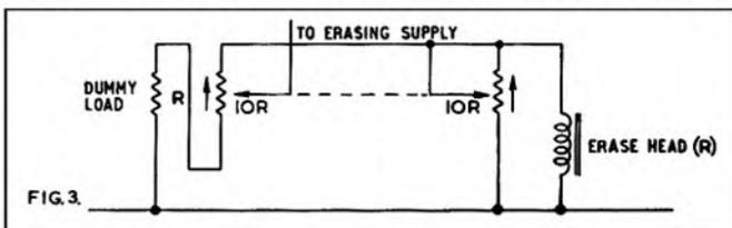
series with the Erase Head to reduce further the power supplied to it. A double-gang potentiometer is used again in fig. 3. This time it is wired to ensure that no power can reach the erase head in the "off" condition because it is shorted out.
