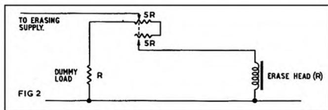
switch with a variable control, the programme material that has already been recorded can be faded in and out as required. This means that, with a little practice, the operator can perform some of the functions of the recording gain control *after* the recording has been made.
