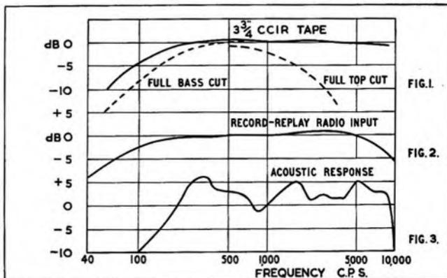
Fig. 3, and shows that the acoustic response over the middle and high frequency range is level within  $\pm 3$ dB limits from  $200$  c/s to  $8,000$  c/s. If you are not used to assessing speaker responses this may not look very impressive, but, in fact, for a cabinet this size the response is remarkably good. It is a sad fact that to reproduce
