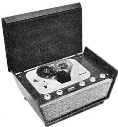
**Manufacturer's Specification:** Garrard magazine loading deck. Tape speed:  $3\frac{1}{2}$  i/s. Spool size: 4 in. or magazine-type. Magic eye level indicator. Built-in microphone. Facilities for mixing and straight through amplification. Size:  $18\frac{1}{2} \times 11\frac{1}{2} \times 8$  in. Weight:  $27\frac{1}{2}$  lbs. Price £40 19s.
