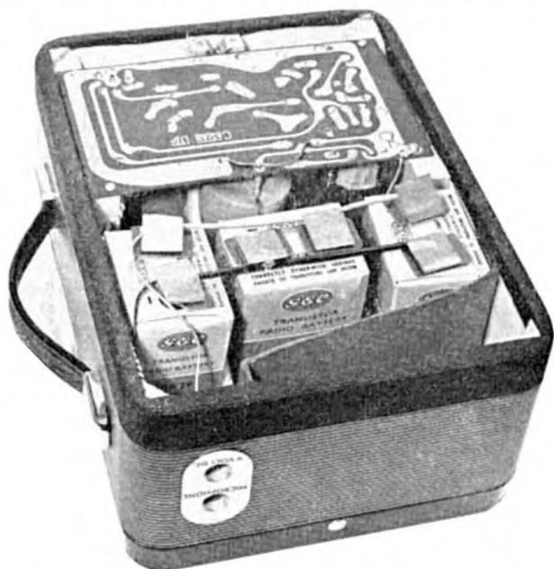
Rear view, with back removed, showing the printed board, batteries, and microphone storage compartment.
