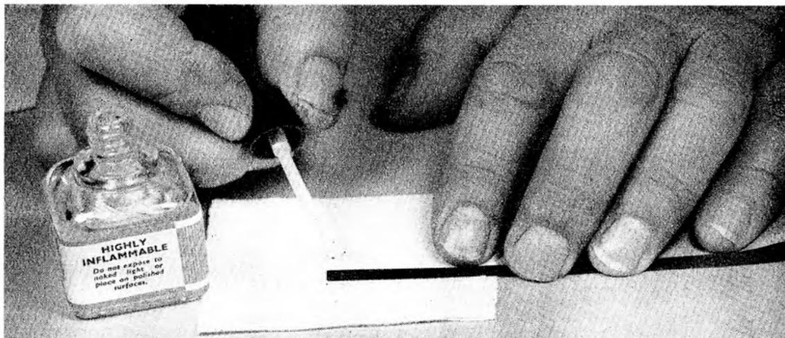
**I**n the previous article I dealt with editing and the splicing of tape using a pressure adhesive jointing tape. It was explained that this type of joint is of a temporary nature, since it can if necessary be taken apart and then remade without damage to the recorded material. However, there is another method type which can be used—the permanent joint—so called since once it has been made there is no way of taking it apart without damaging the tape.
