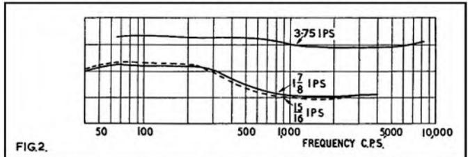
**Playback response:** The top curve of fig. 2 shows that a 200 microsecond C.C.I.R. test tape plays with a level response. This means that British or American pre-recorded tapes will play back with a wide and level frequency response. The same test tape was played at half and quarter speed to give the equivalent of 400 and 800 microsecond recording characteristics. This was
