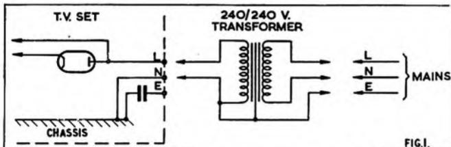
A 1:1 isolating transformer should be used on AC/DC equipment.
