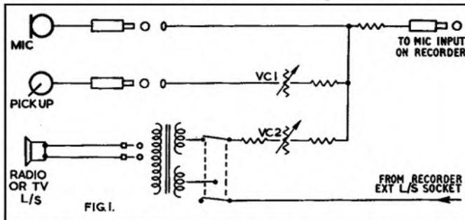
circuit (fig. 1) but it will help to explain the mixer's operation in more detail. You will see that the *microphone* is permanently wired through to the tape recorder, so long as it is plugged into the Tape Mixing Ade, and the only control of its volume is that in the recorder itself.
