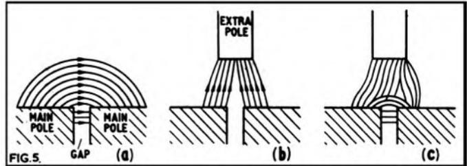
Fig. 5. Flux pattern in a Cross-Field Head. (a) Diffuse field due to main poles. (b) Cross field between main and extra poles. (c) Resultant concentrated field.
