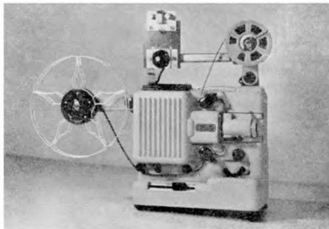
Stage 1. Setting up. The head unit is clamped to the supply reel arm and the film threaded in the usual way.
