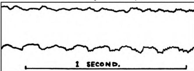
Fig. 1. Fluttergram readings (top) .12% (bottom) .22%
