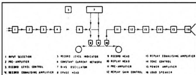
A Block Diagram of the Complete Tape Recording Process
