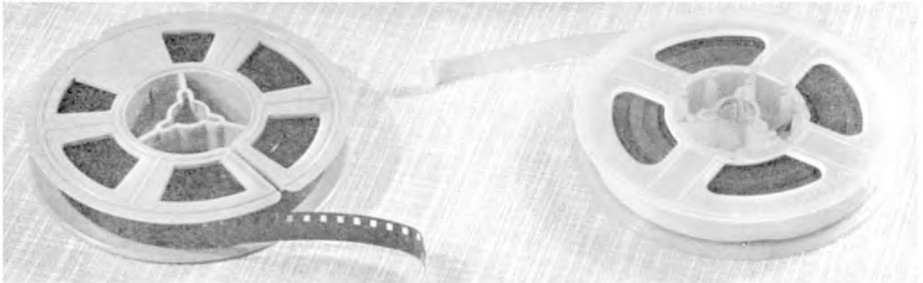
The film (left) is a normal camera loading, slit and spliced at the processing plant to give a standard 50 ft. 3 in. reel with a showing time of 4 minutes. The tape (right) is also contained on a matching 3 in. spool, but due to the thinner base, 150 ft. of standard play tape can be accommodated. The end of the tape leader is rolled and bound with splicing tape for anchorage purposes.
