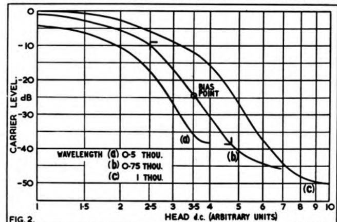
Fig. 2. Transfer characteristics of Carrier-Erase Recording. Carrier level vs head d.c., wavelength as parameter. (0.75 thou' is equivalent to 10 Kc/s at  $7\frac{1}{2}$  i/s, for example.)
