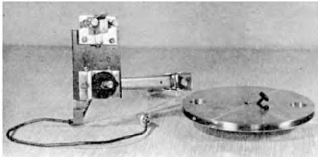
The hardware: The flywheel cum tape spool (right) measures 5½ in. in diameter, weighs 1 lb. and carries a ¼ in. by ¼ in. slot on its outer rim to hold the tape. The head unit (left) is made up from standard "Portable Recorder" kit items. The magnetic head, head plate with tape guides and pressure pad, together with the supply reel spindle and bracket, are mounted on a platform with a means of clamping to the supply reel arm of the projector.
