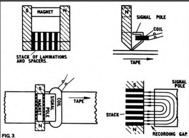
Fig. 3. Recording Head for Boundary-Displacement System. The magnetic circuit through the high-reluctance lamination/spacer stack is shunted by the adjacent signal pole, each half carrying flux in opposite directions with a neutral point in the centre, thus: Energising the signal pole produces a uniform field component which adds to one half of the standing field and subtracts from the other, thus shifting the neutral point from the centre.
