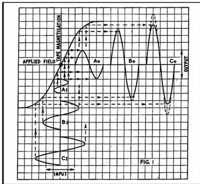
Fig. 1. Heavy curve at top left shows magnetisation curve (transfer characteristic) of A.C. biased tape. Input waveforms A, B, C result in output waveforms A, B, C. Peak distortion suffered by B and C; dashed "caps" show correct waveform peaks in absence of transfer characteristic curvature. B corresponds roughly to "maximum" modulation for 5 per cent. 3rd harmonic distortion in input; A about -8dB, C about +3dB on this.
