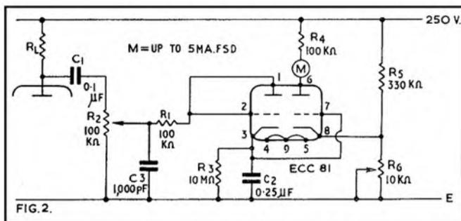
but the diode is reversed.  $R_1$  will now feed to pin 3 and pins 1 and 2 will connect to  $R_3$ .  $R_5$  has to be adjusted for zero, which will be *maximum* current through the meter, maximum signal will reduce the current to zero. Hence the meter can never be overloaded.
