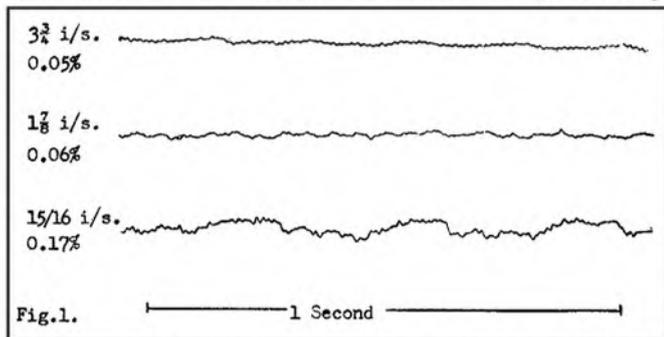
is important. The frequency response at  $1\frac{7}{8}$  i/s is comparable to that of most  $3\frac{3}{4}$  i/s recorders, and half track gives excellent signal to noise ratio and freedom from tape edge effects. At  $3\frac{3}{4}$  i/s musical quality is quite a revelation, and the very low speed of  $15/16$  i/s is perfectly satisfactory for good quality speech or dictation recording.
