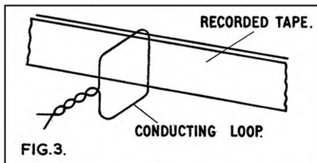
thin compared to the spacing of the magnet poles on the tape the e.m.f. generated by the loop  $E = vwB$  where  $v$  is the speed of the tape,  $w$  is the width of the tape and  $B$  is the surface induction of the tape at the frequency under test.
