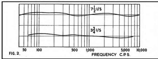
$7\frac{1}{2}$  i/s and once per second at the lower speed; this proved to be due to a slightly eccentric pressure roller. It can be distinguished on the bottom fluttergram for the  $7\frac{1}{2}$  i/s test.
