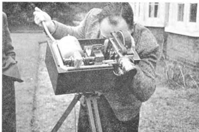
Camera set-up showing the lower half of blimp with *Parvalux* motor and gearbox.
