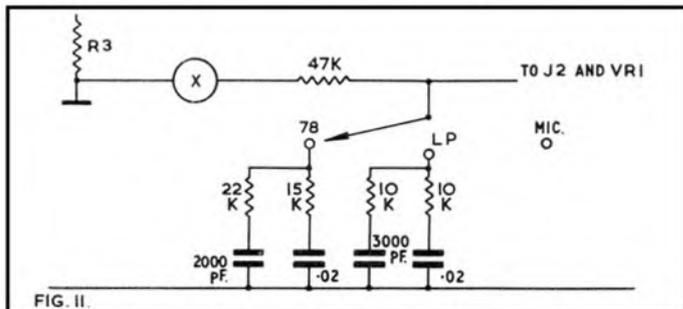
Fig. 11. A suggested lossier equalising circuit.
