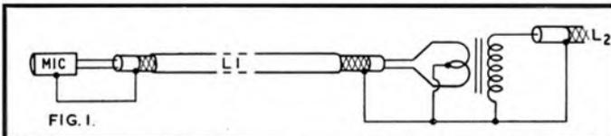
is twisted and the microphone case is left disconnected, but it must not go near to electrical fittings, earthed pipes, or wet grass etc., or the balance may be upset and hum result.
