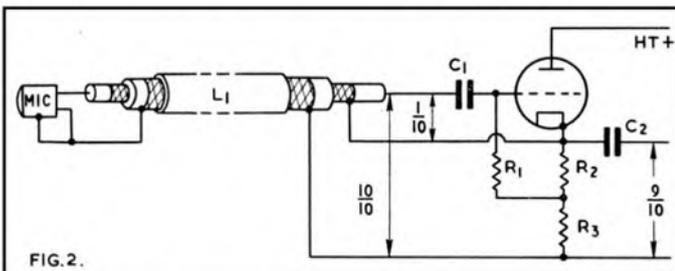
have to be DC too) to the valve. This is the usual arrangement with the expensive professional condenser microphones.
