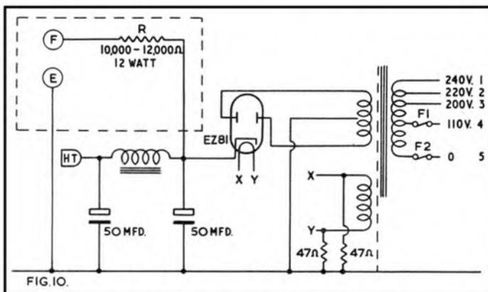
Fig. 10. Circuit of a suitable power pack.
