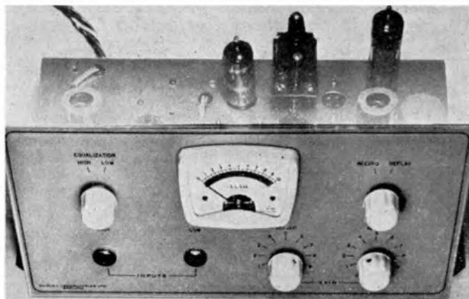
difficult, given suitable heads, to achieve 60 c/s to 15,000 c/s at  $7\frac{1}{2}$  i/s, and 60 c/s to 9,000 c/s at  $3\frac{1}{2}$  i/s  $\pm 3$  dB. Unfortunately, it is even less difficult to achieve equal or even more exaggerated distortion and noise figures at the same time.
