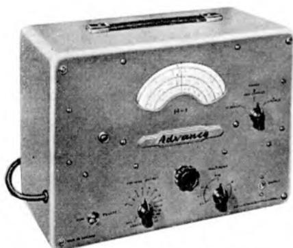
An Audio Signal Generator may be a beat frequency oscillator or a resistance/capacitance phase shift oscillator. The B.F.O. offers the considerable advantage of covering the whole audio range in one sweep, but the phase shift type is generally more accurate for a limited outlay.
