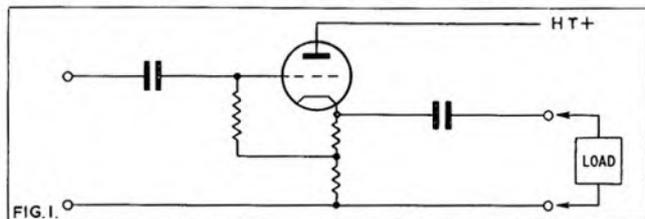
to all sorts of circuits without upsetting them. B. Its output impedance is very low, even below 100Ω, with a suitable choice of valve. This is perhaps its most useful property as long leads can be run from it with much less fear of introducing hum or losing the high frequencies in a long screened lead as with high impedance circuits. It is also possible to use a wide range of loads without altering the output voltage—provided such loads
