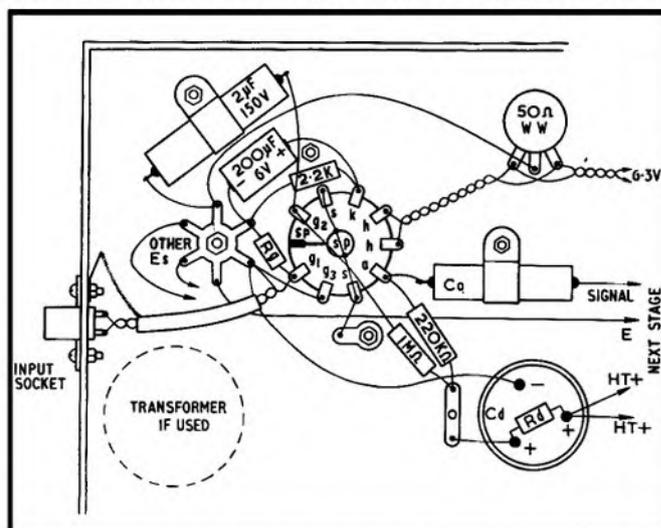
**Fig. 2.** Layout for EF86 input stage using anti-microphonic holder (with normal holder the screws come opposite sp and h pins, in which case use sp for earthing instead of s). See Fig. 3 for circuit.
