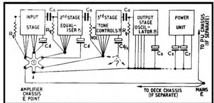
Fig. 4. Principles of earth wiring of amplifier in simplest form; see text for details. Cs = smoothing capacitor, Cd = decoupling, Cr = reservoir.
