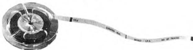
A USEFUL new accessory was announced recently by *Zonal* that, amongst other things, will provide an inexpensive, accurate way of determining the exact running speed of a tape recorder. The whole length of the tape is divided into sections exactly  $7\frac{1}{2}$  ins. long. Thus a known number of sections can be spliced into a tape and the precise speed calculated. It is marked for identification purposes and can be used as leader tape.
