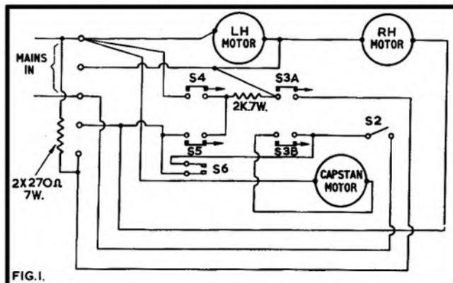
Check that this is correctly tensioned for positive action before investigating supposed switch faults. These switches bring the capstan motor into operation and shunt R1 across the feed-spool motor for reduction of torque; the two spooling motors then being in series, across the supply.
