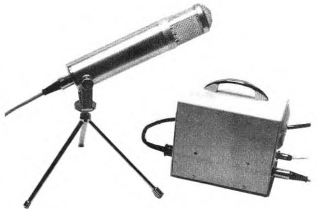
**4.** Here is the finished job. It looks good and it is good. The construction of the microphone/pre-amplifier unit demands really clean, careful work. The foil diaphragm is now supplied in finished, capsule form, thus obviating the most delicate work. Total time taken was 10 hours.
