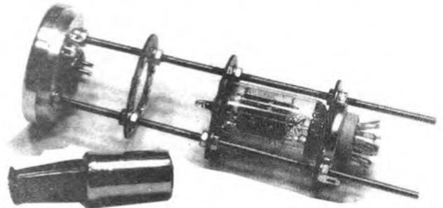
**5.** This stage shows the mic/pre-amp unit completed mechanically and ready for wiring. The only "tricky" work is in the first step, with soldered joints to the 5-pin base plug. See photo 7 opposite.
