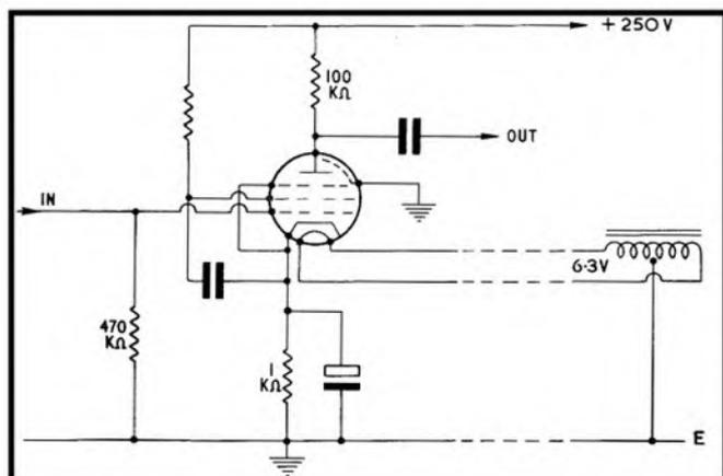
**Fig. 1.** Average working conditions for EF86 voltage-amplifier valve. Quoted hum figure is  $1 \mu V$ , and general noise  $2 \mu V$  in the band 20-10,000 c/s, expressed as equivalent grid input and due to valve alone.
