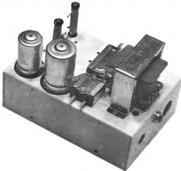
**3.** The power pack chassis, shown here, has been fitted with all the components that can be mounted without preparation. The items in photo 2 are then added and the unit is completed with very little wiring.
