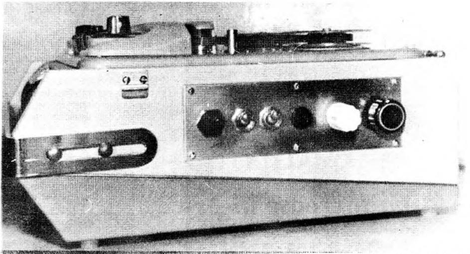
head and unscreened to the phones and battery. A tape should be played back through the phones and the third head roughly aligned by ear for maximum signal. Some hum may be noticeable. This will be due to the long leads employed for the temporary connections.
