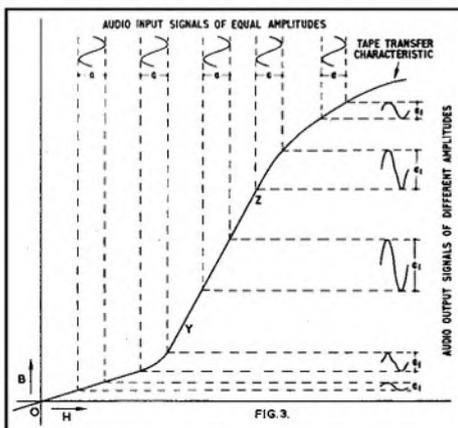
**Fig. 3.** This shows how the output level varies according to the operating position on the curve.
