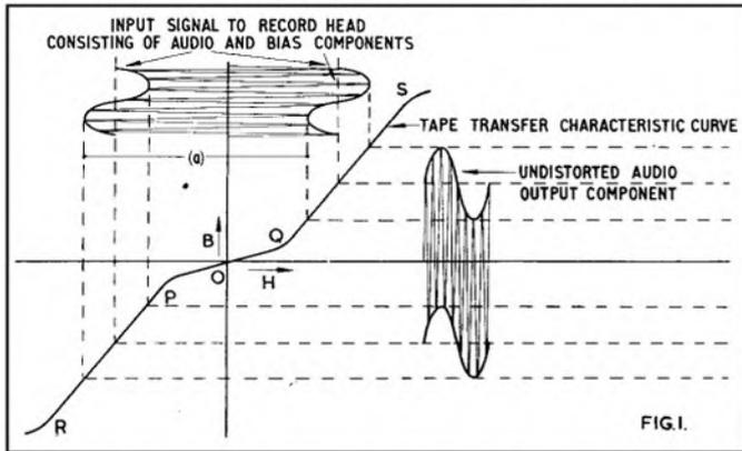
**Fig. 1.** This shows the normal optimum bias arrangement, where **B** is the magnetic flux density in the tape coating, **H** is the magnetising field applied by the record head, and (a) is the peak-to-peak amplitude of the bias voltage.
