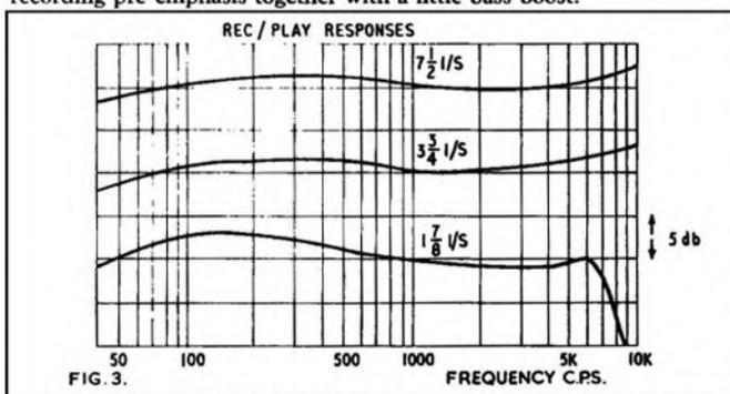
Fig. 3 shows the overall record-replay responses—radio input to line output via the diode socket. These responses were taken at 6 dB below test-tape level to allow for the severe high note pre-emphasis used when recording 50, 100 and  $200\mu\text{s}$  time constants at tape speeds of  $7\frac{1}{2}$ ,  $3\frac{3}{4}$  and  $1\frac{7}{8}$  i/s, respectively.
