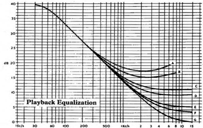
quality replay head, having a gap of 3 $\mu$  (0.12 thou.) will therefore require an additional high frequency lift to maintain the desired replay characteristic. The amount of high frequency lift is not great (approximately 3 dB at 10 Kc/s) and would take the shape shown in the curves A and B of the graph.
