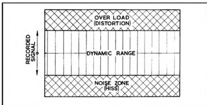
**Fig. 1.** The beginner soon finds that if the recording level is too low background 'hiss' is troublesome, while if it is too high overload distortion is present on peak signals. The ideal is to arrange the controls so that the signal operates within the 'sandwich' shown here.
