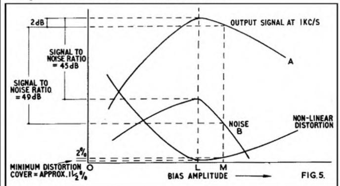
Fig. 5. With a bias current level L signal-to-noise ratio is 45 dB, and distortion is about 1½%. If the bias current is now increased to M, the signal-to-noise ratio improves to 48 dB, while the distortion becomes very slightly worse (around 2%).
