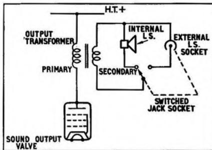
**Fig. 1.** This diagram shows how a switched jack socket can be wired to the loud-speaker circuit so that when the plug carrying the external speaker is inserted the internal speaker is automatically switched out of circuit.
