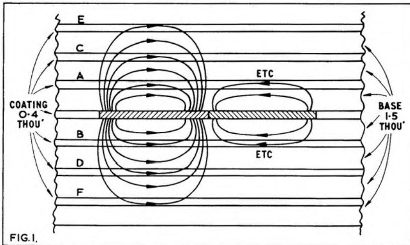
This shows adjacent layers of tape on a spool with two half-wavelengths of master signal (recorded 500 c/s at  $7\frac{1}{2}$  i/s) to scale, and flux lines passing through other layers, not necessarily to scale.
