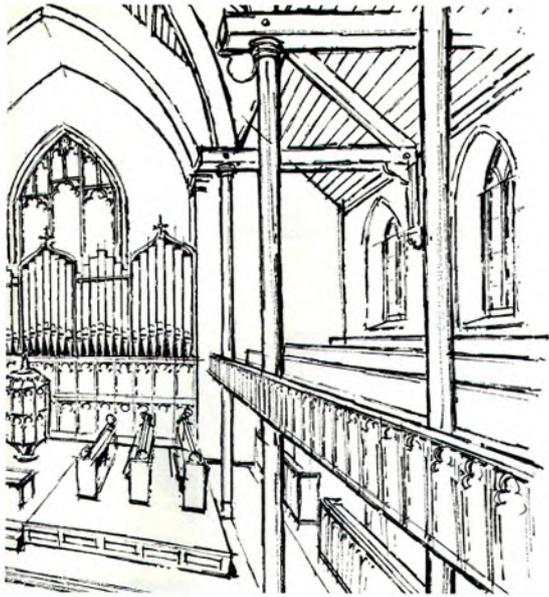
**Fig. 1:** This type of church is seen in practically every town. Provided the roof timbers and projecting galleries don't result in a too-short reverberation period, this layout gives excellent balance and blend.
