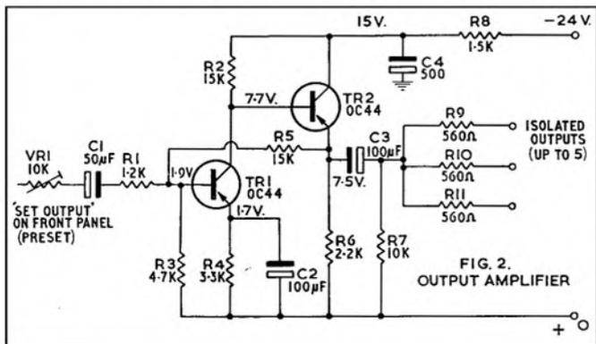
expensive silence! The voltages on the circuit diagrams can be checked against the values actually obtained. For this, any instrument will be satisfactory since the circuits are low impedance and will not be unduly loaded.
