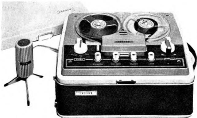
Full facilities for  $\frac{1}{2}$ -track recording and replay, as well as MULTIPLAY and inter-track recording, are offered by the CR1607 (shown with microphone), with speeds of  $3\frac{1}{2}$  and  $1\frac{1}{2}$  i/s. Peak-to-peak wow and flutter figures of 0.6% are claimed, with a frequency response from 80 c/s to 15Kc/s at the faster speed and 80c/s to 10Kc/s at  $1\frac{1}{2}$  i/s.
