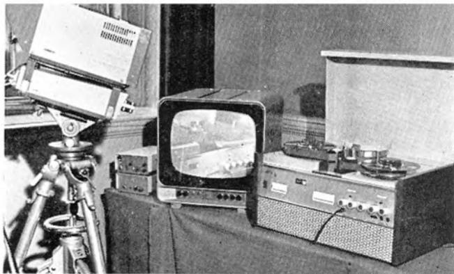
Coupled to its pre-amplifier by a rotating transformer, the head scans 1in. tape moving at  $7\frac{1}{2}$  i/s, at approximately 23 yards per second. Maximum playing time, using 1,800ft. of LP tape, is 45 minutes.
