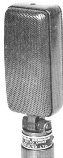
**Manufacturer's Details:** High quality ribbon microphone manufactured to broadcasting standards. Frequency response:  $\pm 3$  dB, 30 c/s to 16 Kc/s. Field of pick-up: figure of eight, unless modified by acoustic correction pads. Sensitivity: 58 dB below 1V/dyne/cm<sup>2</sup> at 40 K ohms. Impedance: 30-50 ohms. Finish: satin chrome overall. Price: £15 15s. Manufacturer: Reslosound Ltd., 24 Upper Brook Street, Mayfair, London, W.1.
