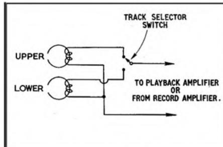
Fig. 6. Typical  $\frac{1}{2}$ -track head switching arrangement.
