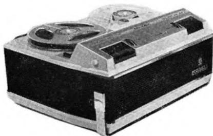
**F**OUR new recorders have been added to the *Grundig* range—Models *Luxus TK 14L, TK 17L, TK 18L* and *TK 23L*. Common specification points are tape speed -  $3\frac{3}{4}$  i/s; frequency response - 40 c/s to 12 Kc/s  $\pm 4$ dB; wow and flutter -  $\pm 0.2\%$ ; output power - 2.5W; dimensions -  $13\frac{1}{2} \times 10\frac{1}{2} \times 6\frac{3}{4}$  in.; weight - 22lb. All four incorporate high impedance and external speaker outlets and all are mains powered.
