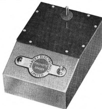
**V**ARYING in price from £6 5s. to £15 10s., a new production of Harvey Erasers was recently announced. Twelve models are now obtainable, to handle spools of up to 12in. diameter and tape widths up to 1in. The units can also be used to demagnetise small metal objects such as watches and tape heads. In the latter case, care should be taken to protect loudspeakers magnets.
