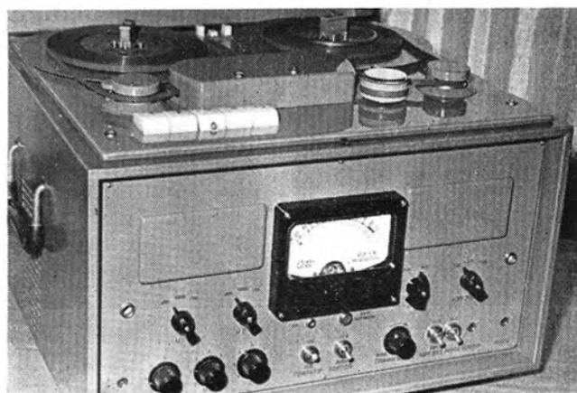
phone, radio receiver and gramophone. One motor is used for track switching. Double-purpose amplifiers and dual-purpose heads are used for recording and playback. The recorders can be powered from an AC mains supply and have two loudspeakers.
