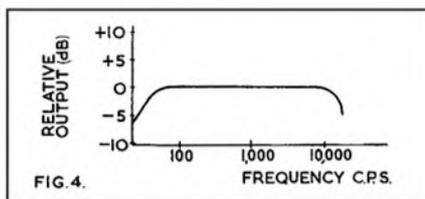
FIG. 4. Output obtainable from a tape head amplifier by modifying equalisation at turnover frequency
