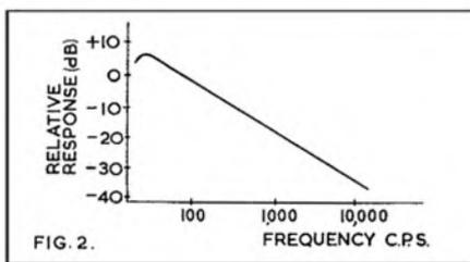
FIG. 2. Amplifier response needed to combat 6dB/Octave effect
