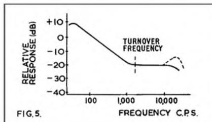
FIG. 5. Output shown in fig. 4 can be obtained from head amplifier with this equalised response
