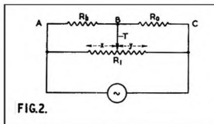
Bridge circuit illustrating theoretical arrangement of motors and control potentiometer
