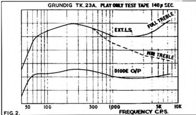
was obtained with the tone control at maximum top cut. It will be seen that the playback characteristic closely conforms to the now common DIN and CCIR 140µ S time constant. Identical responses were obtained on the top and bottom tracks.
