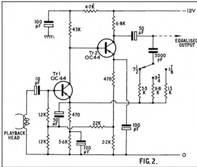
LAST month we saw the need for playback equalisation. We saw that the EMF induced into the playback head winding rises constantly at 6dB per octave up to the turnover frequency, at which point the EMF commences to drop slowly at first and then fairly rapidly. Previous articles in this series have shown why this happens.
