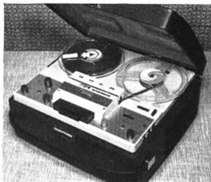
which is illustrated overleaf, is a vernier control set in the head cover with which the playback head azimuth can be altered. Microphone input characteristics are 0.15mV at 5K (for 1 Kc/s), terminals for one stereo or two mono microphones being included. Radio and
