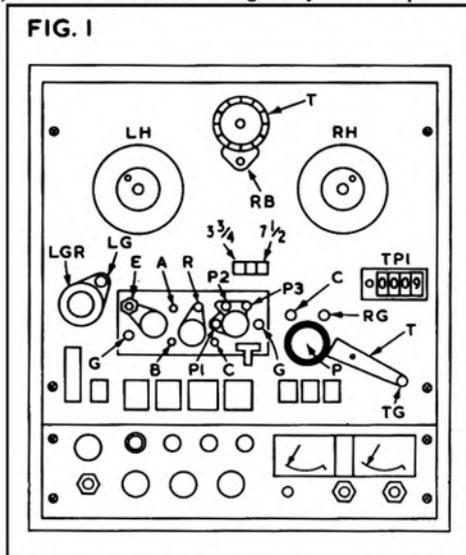
Front panel with head cover plate removed. LH—feed reel. RH—take-up reel (both with plain spindle and key locator). T—timer dial. RB—reset button. LGR—left guide flywheel. LG—left guide. RG—right guide. C—capstan spindle. P—pinch roller. T—tension arm. TG—tension arm guide. TPI—digital tape position indicator.
