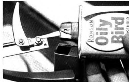
type of grease would be suitable, but with the same property. In each case, it is essential that the property is not lost with movement and heat. The answer is a lubricant with an oxide inhibitor, and with this clinging property 'built-in'.
