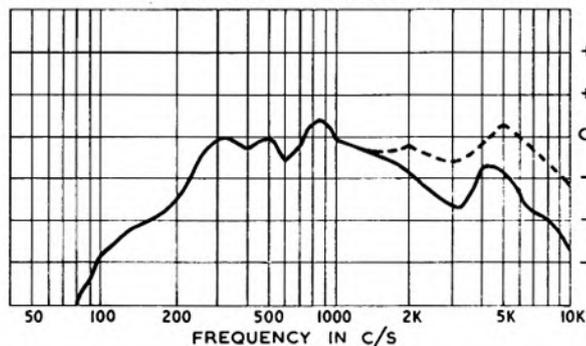
FIG. 5 GRUNDIG GDM 311 MICROPHONE RESPONSE
