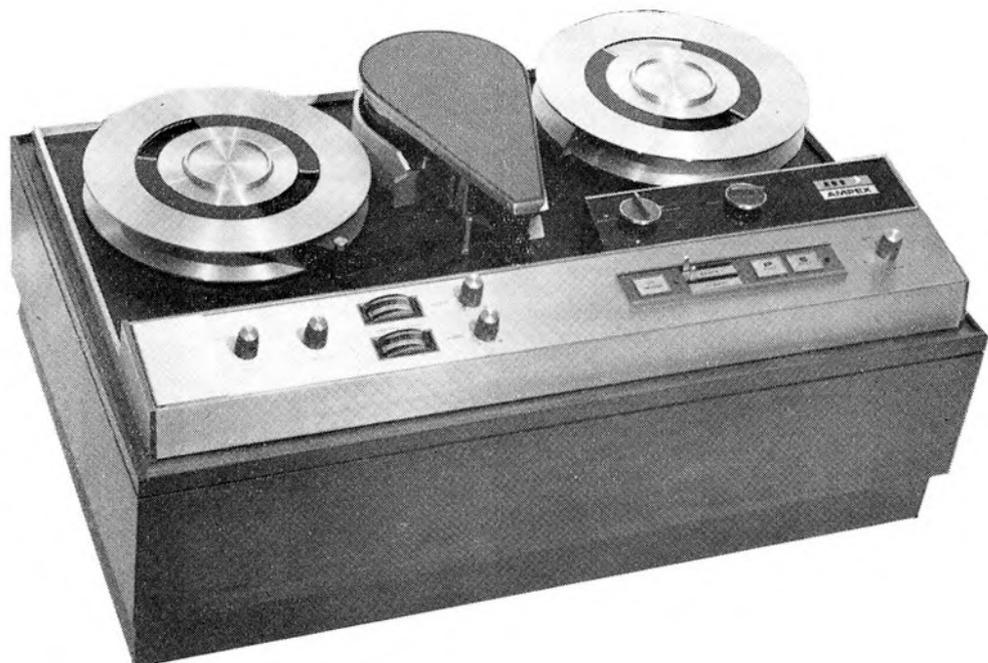
**Right:** Ampex HVR helical-scan recorder operates at 9.6 i/s.
