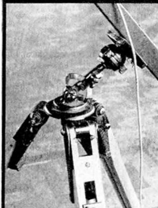
**Left:** Swivelling pillar and ball joint of ex-army tripod.
