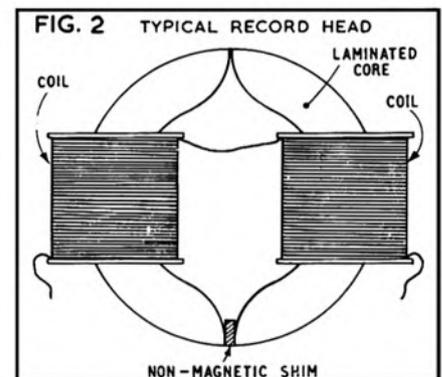
head for both recording and reproduction and a second head for erasing. A section of a typical head is shown in fig. 2. It consists of a laminated coil of some such material as *Permalloy*. This has a very narrow hysteresis loop, which means that it can be magnetised with ease but loses its magnetism immediately the magnetising field is removed. Narrow gaps at each end of the core are filled by non-magnetic 'shims' and on each side a multi-turned coil is wound.
