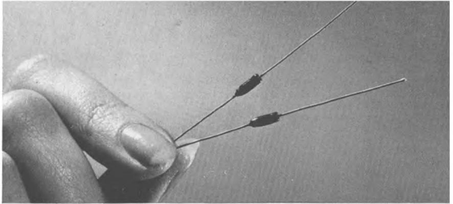
When the external polarity is reversed, the potential barrier, instead of being neutralised and eventually destroyed (temporarily of course), is reinforced. This is because the external potential adds to the potential of the barrier, as shown in fig. 5.
