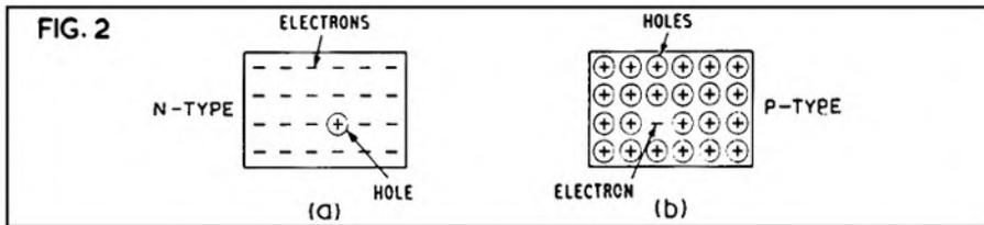
electrical charge of a hole is exactly equal in magnitude, though opposite in sign, to the charge of an electron, and that there exists a mutual attraction between holes and electrons. A process upon which the operation of a semi-conducting device is based is called *recombination*. This happens when an electron fills a hole, after which neither the hole nor the electron can further contribute towards the conduction of electric current.
