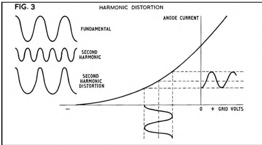
Harmonic and amplitude distortion are two more forms of distortion which are produced by curvature of the amplifier characteristic. Even the 'straight' portions of most amplifier characteristics have a certain amount of curvature. The pentode valve is a particularly bad offender in this respect.
