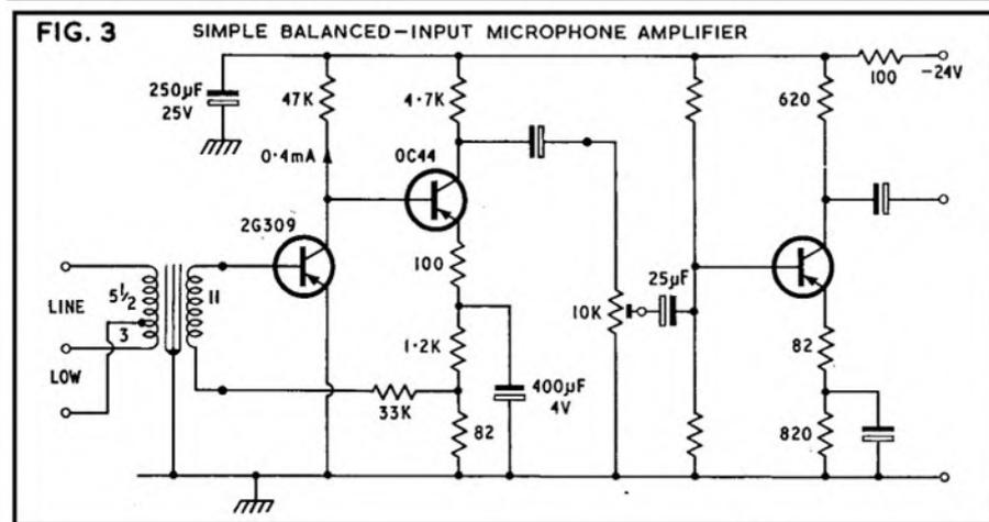
amplifier. The circuit has been somewhat experimental in nature, but the results are quite reasonable within the limits set by economy, and one amplifier to this design has been in the mixer now for a while; no performance measurements have been made, but when used with an inexpensive moving-coil microphone the emerging sound is quite reasonable, which was after all the basis of the design philosophy for this amplifier.
