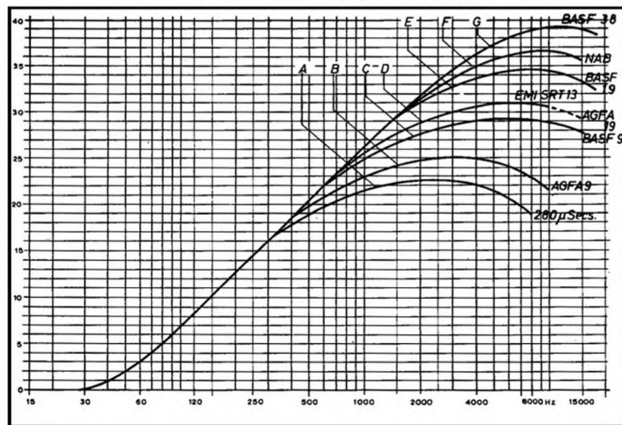
Fig. 1 Unequalised output from Standard Test Tapes.
