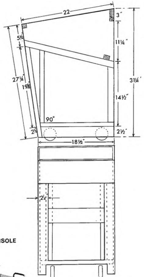
FIG. 7 CONSTRUCTION OF CONSOLE
