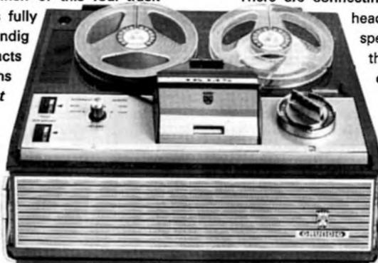
There are connecting sockets for recording/playback, monitor headphones and switchable extension loud-speaker. There's even a press-button reset for the position indicator! And—to guarantee cool operation over long periods of playing and recording, the TK145 has the exclusive Grundig single-unit combination of motor and mains transformer.
