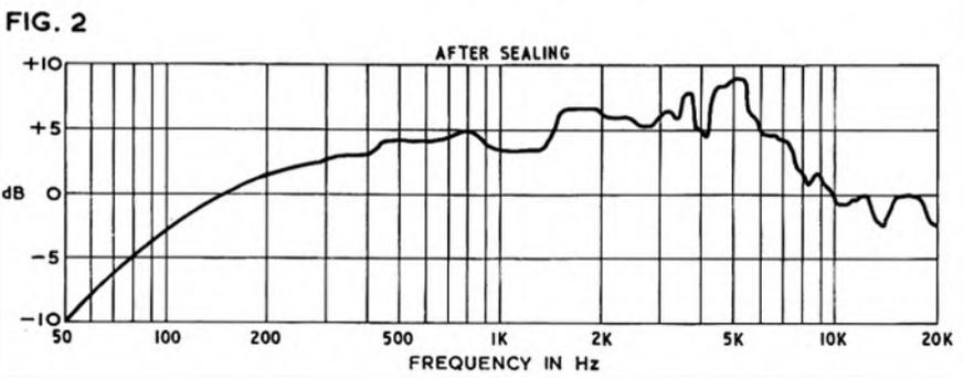
is seen to be substantially flat from 100 Hz to 20 kHz apart from the slight roll off below 100 Hz the overall performance is better than that claimed by the manufacturers. When used in the hand, or as a neck microphone, it is insensitive to external noise, and speech is clear and crisp. For music recording some degree of bass lift may be necessary.
